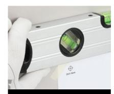
Place template on wall with tape. Make sure that template is level. Mark the hole locations.
