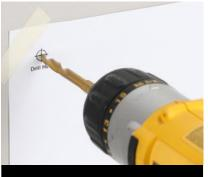
Drill with a 1/4" diameter cobalt drill bit.
